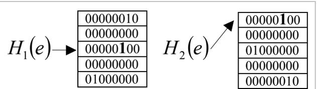
Figure 7: As before, suppose flow  $e$  is to be forwarded to interface 2. Now, let us suppose that  $H'(e) = 3$ . So,  $j = (i + H'(e)) \bmod I = (2 + 3) \bmod 8 = 5$ .
