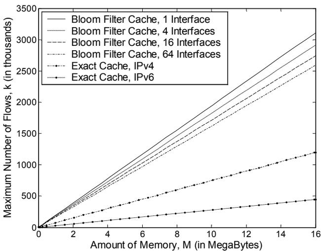
Figure 6: Effect of storing routing information on effective cache size,  $p = 1e-9$ , using optimal Bloom filter dimensions
