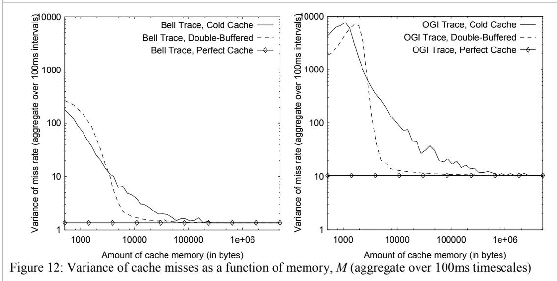
Figure 12: Variance of cache misses as a function of memory,  $M$  (aggregate over 100ms timescales)
